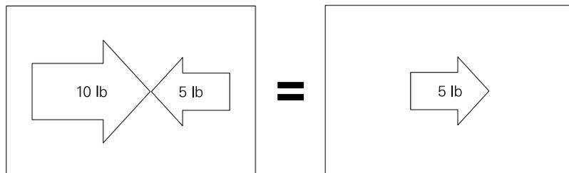
If 10 lb of force were applied equally in both directions, the net force would be zero and the object would not move.
