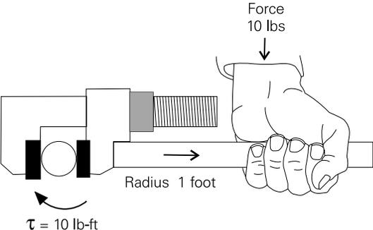
An increase in force or radius would result in a corresponding increase in torque. Increasing the radius to 2 feet, for example, results in 20 lb-ft of torque.
