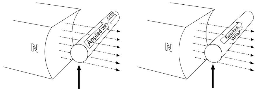
The amount of induced CEMF depends on many factors such as the number of turns in the coils, flux density, and the speed which the flux lines are cut.
