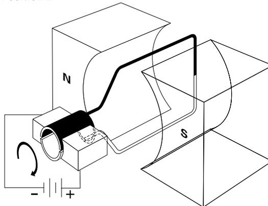
As the conductor continues to rotate from position 2 to position 3 current flows away from the commutator in the white half and toward the commutator in the black half. Current has reversed direction in the conductor. This is known as commutation.
